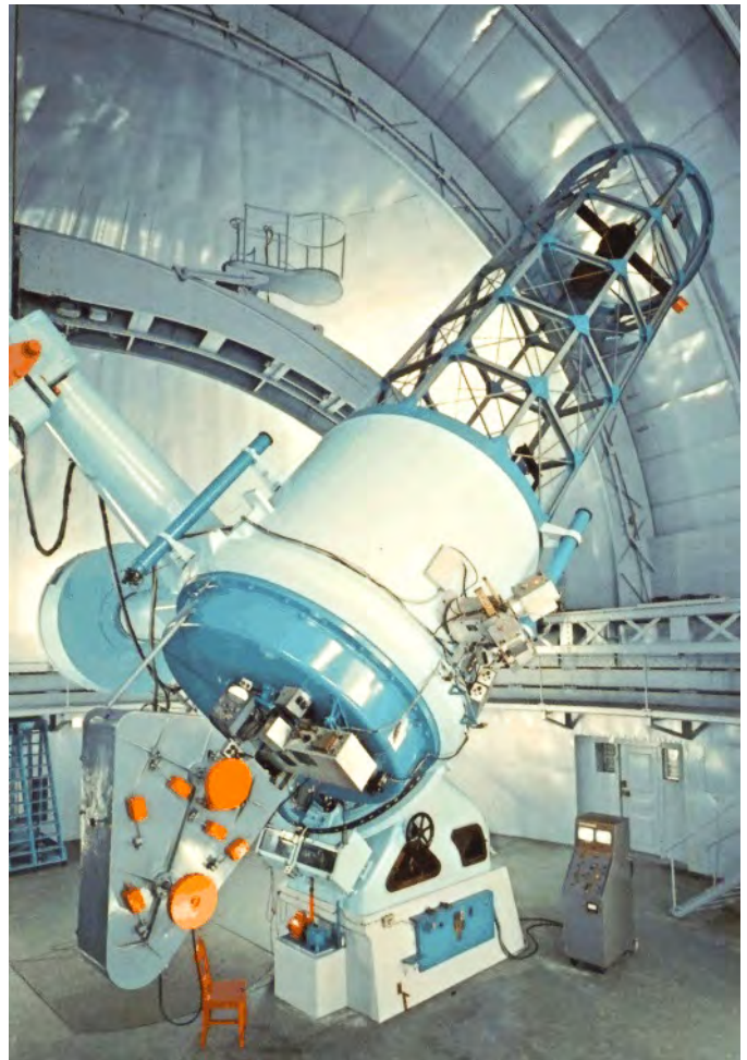
Figure 1 — The three main components of the close-binary radial-velocity program belonged to three generations of astrophysical instruments: (1) The telescope — representing the 1930’s technology — utilized the first fused-Pyrex mirror, but was long and subject to large mechanical stability issues. (2) The Cassegrain spectrograph (the semi-triangular structure, with red-painted counter-levers, below the main-mirror cell) was designed in the 1960s with high efficiency in mind as an all-reflection instrument. (3) The CCD detectors reflected the 1990s technology with quantum efficiency exceeding 80%; they were still relatively small in terms of the number of pixels.
