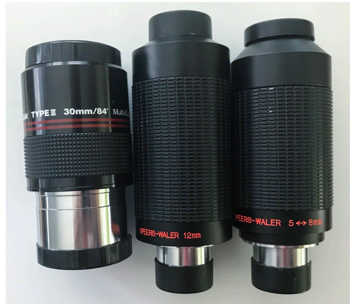
Figure 2 — Used set with a zoom eyepiece— a 30 mm, a 12 mm, and a zoom eyepiece. WALTER = Wide Angle, Long Eye Relief, original design by Glenn Speers of Antares, no longer for sale on the retail market.
