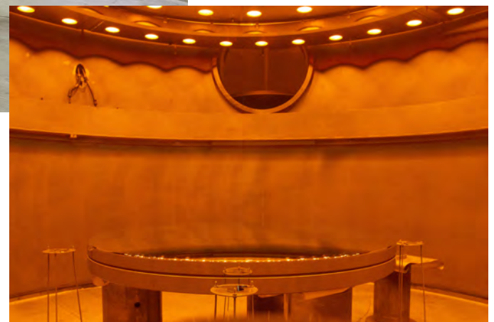
Figure 2 — Inside the CFHT coating chamber post flash.
