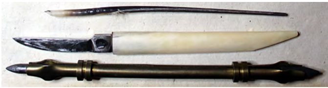
Figure 7 — Reproductions of an 18th-century pen made from a crow quill, a penknife, and a porte-crayon for drawing with a lead. Reproduced courtesy of the Specula astronomica minima .
