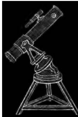
Figure 4 — Diagram of an amateur reflector on a parallactic mount. Sir Adam’s reflector was said to be similarly supported. From John Browning, A Plea for Reflectors (London: John Browning, 1876), p. 15, figure 4.
