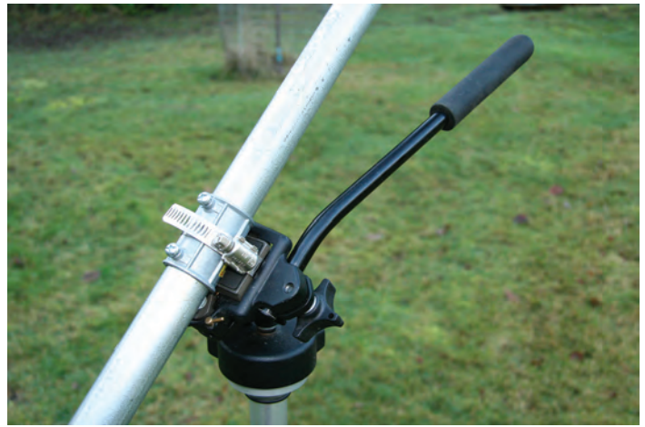
Figure 2 — The coupling sleeve mounted on the video head.
