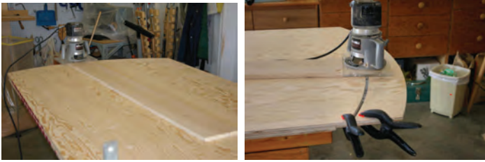
Figure 1 (left) — Cutting the circle template. Figure 2 (right) — Routing ring pattern - base
