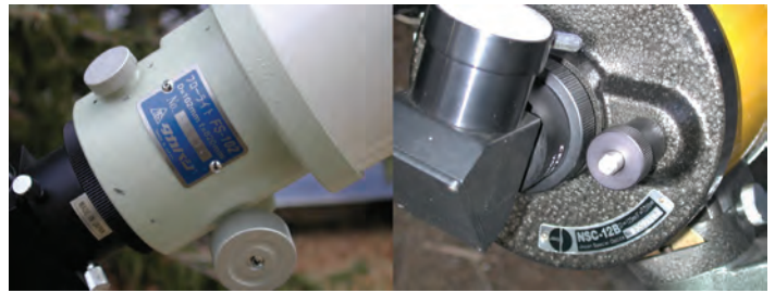
Figure 4 — The old fashioned rack-and-pinion focuser of the Tak was stiff in the cold, while the buttery-smooth JSO focuser had mirror shift.
