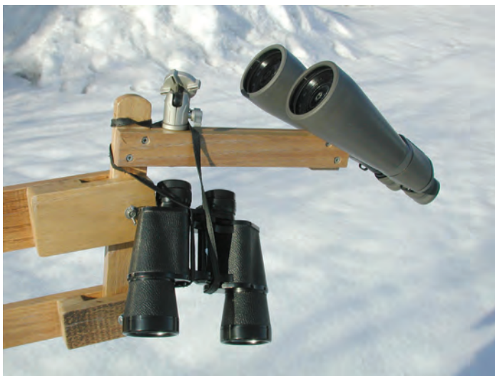
Figure 5 — Economical instruments, including used Nikon 7×50 too old to have a model name, and the ubiquitous 15×70 (these are “Galileo” brand). This combo is more versatile than one 10×50.
