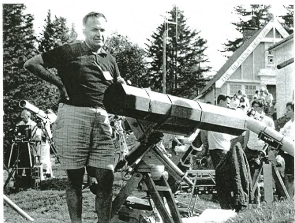
Henri Simard is seen at Stellafane in August, 1967, in a photograph sent by his daughter, Mrs. Martine Normandin. His 6-inch Newtonian was made mostly of plywood, with pipe axles turning in ball bearings.
