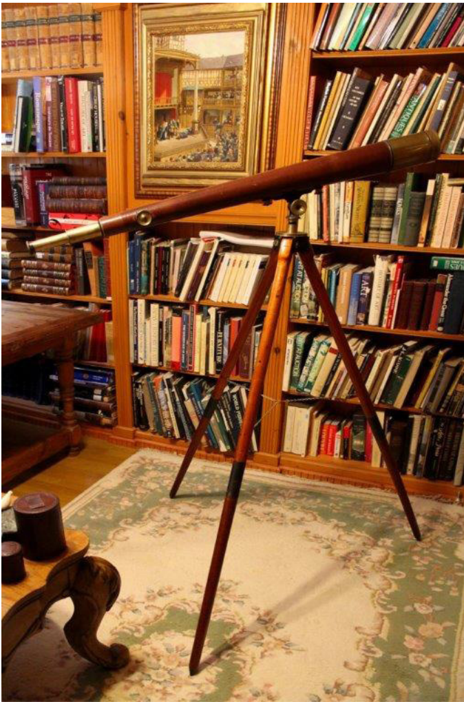
Dollond achromatic refractor (“Outlook” model, 3-inch O.G.), ca. 1910, London. This instrument has a Nova Scotian provenance, and though primarily an instrument for marine or terrestrial use, it is nice to think that it could have been used for viewing the 1910 apparition of Halley’s Comet (1P/Halley) (DTM tba).
