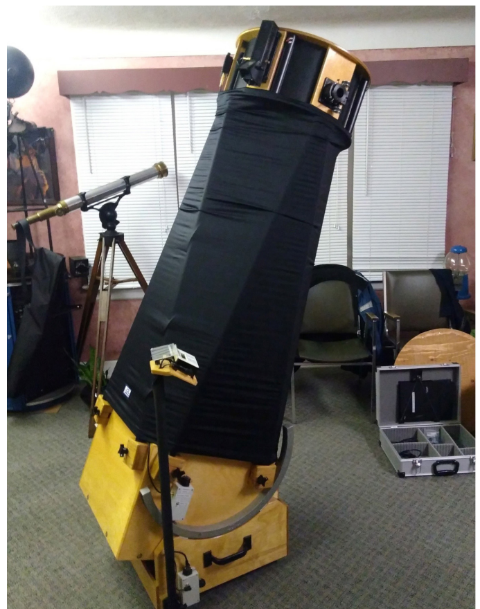
Rebuild around a 17.5 inch Coulter mirror. Photo by Bob Lewis.
