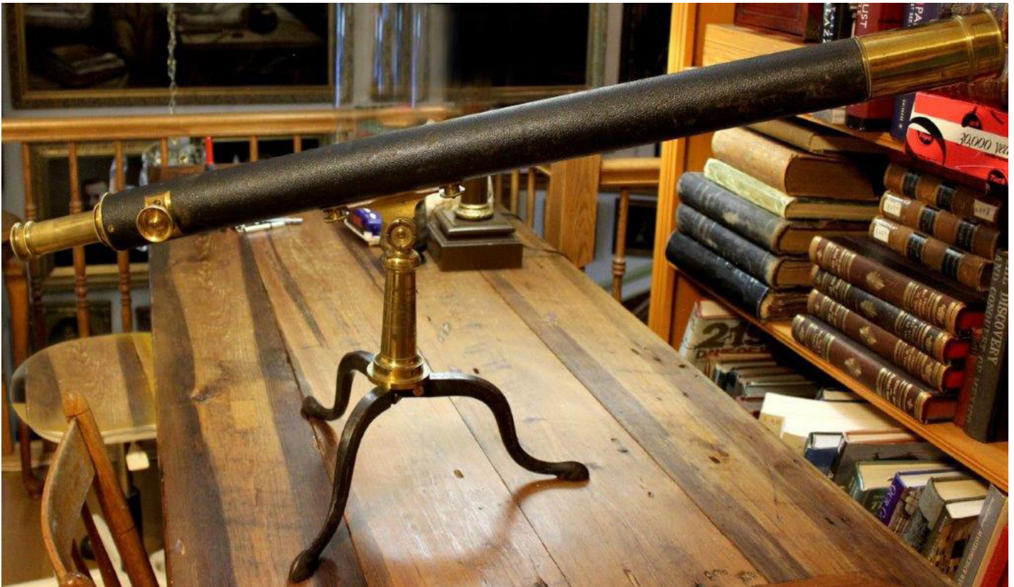
Hearn & Harrison of Montreal (ca. 1880–1930s) achromatic refractor on a library stand, late-19th- early 20th century. These small mounted achromats with object glasses (O.G.) ranging from 40 mm to 90 mm, could be found in amateur hands (DTM tba).
