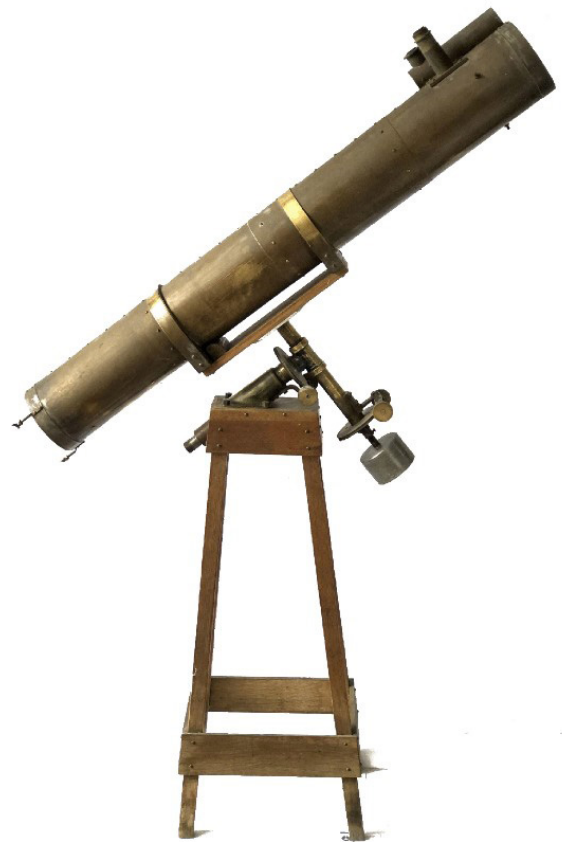
Unsigned, equatorially mounted Newtonian reflector, late-19th- early 20th century (the original 6-inch primary mirror is missing; a replacement has been commissioned). This beautifully made instrument has a provenance associating it with Sir Frederick Banting (1891-1941), one of Canada's first Nobel laureates (1923), although no other evidence has come to light that he had any interest in astronomy (DTM tba).
