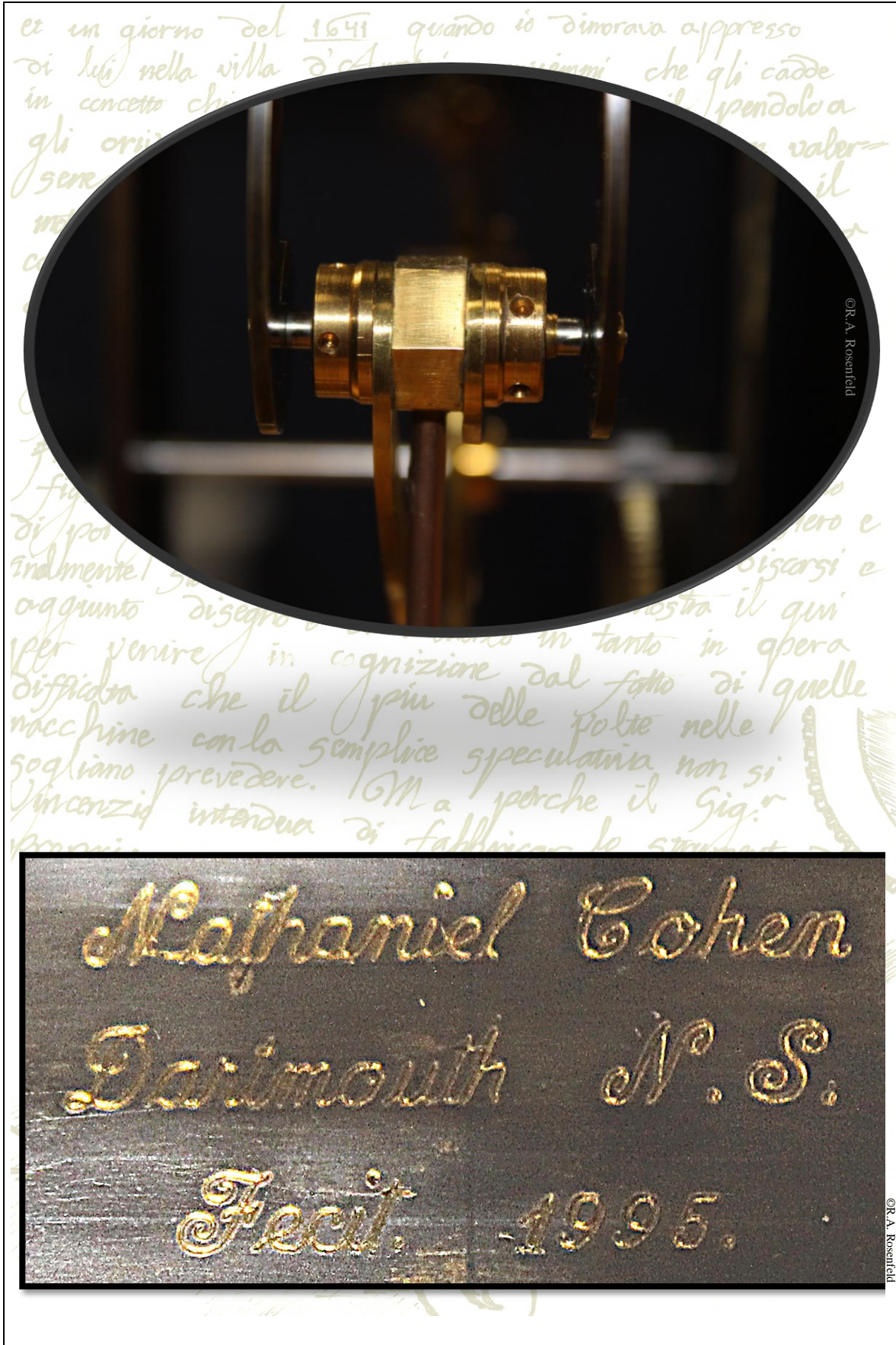
above: suspension bracket & arbor; below: name plate
